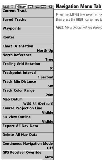
Press the MENU key twice to access the Main Menu System, then press the RIGHT cursor key to select the Navigation tab.
